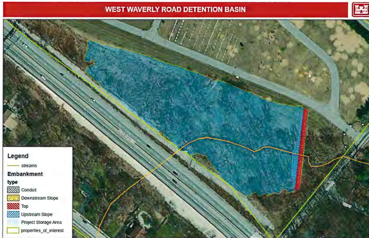
Figure 4. Conceptual design for the proposed West Waverly basin.
